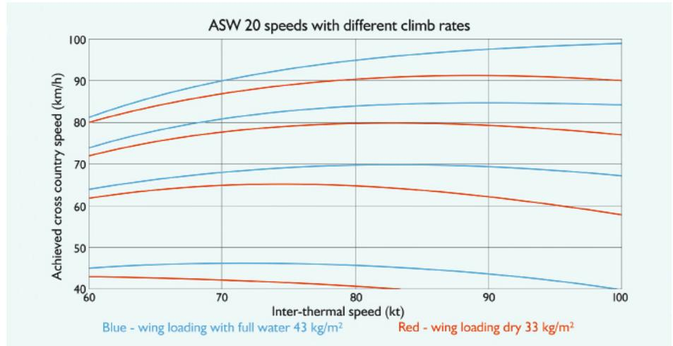
Figure 1: manufacturer's data for an ASW 20 at sea level (Enhanced by Steve Longland)
