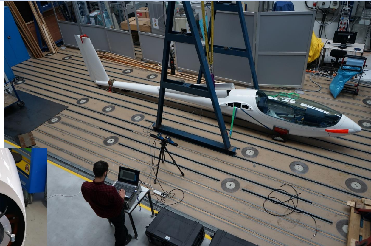
Structural certification tests for motor mounting and battery/REX mounting at DLR Stuttgart
