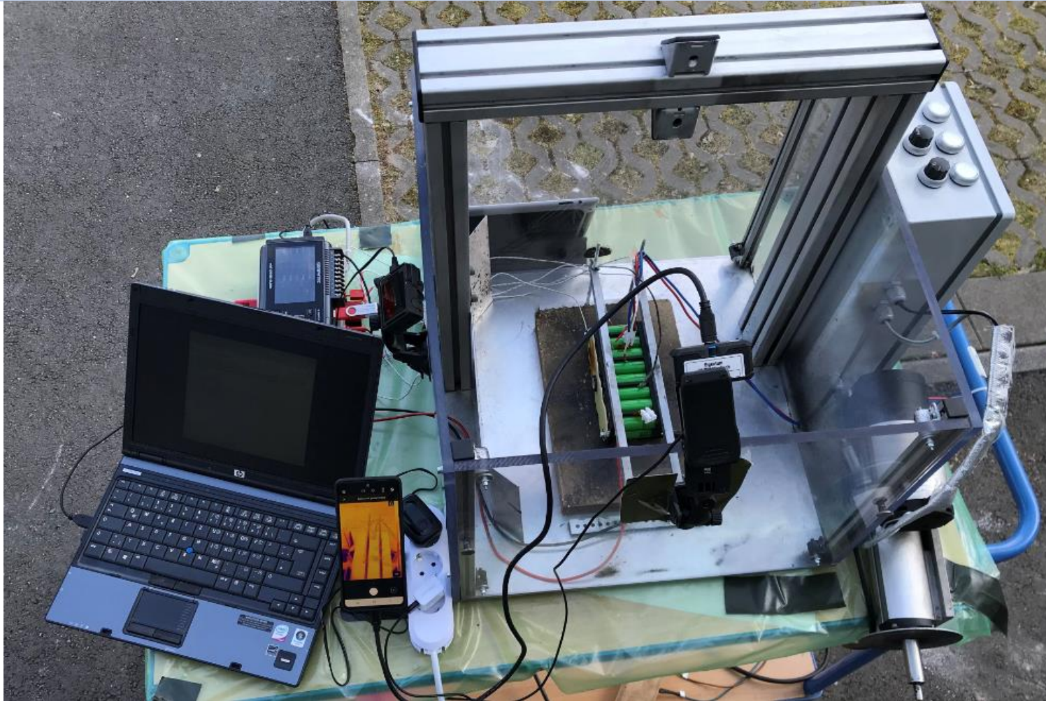
Single 18650 cell with heater coil to drive into thermal runaway
