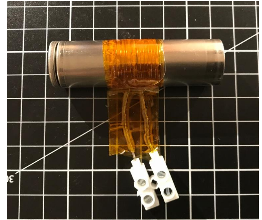
Single 18650 cell with heater coil to drive into thermal runaway
