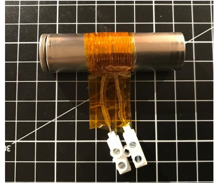
Preparation of single 18650 cell with heater coil to drive into termal runaway
